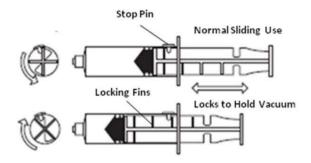
1. Examine the stopcock. The stopcock has two luer connections to attach to the needle and syringe. Air can be exchanged with the stopcock in the open position. The stopcock is open when it is aligned parallel to the syringe; it is closed when perpendicular to the syringe.
